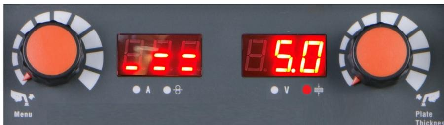
1. Press and holding in the right hand dial until the display changes to material thickness (*as above*).
