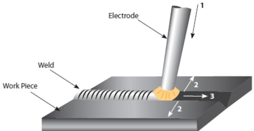
The operator can choose the manipulation of electrode based on welding joint, welding position, electrode spec, welding current and operation skill etc.
