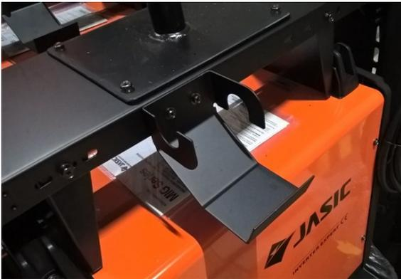
10. Finally locate wire feed unit onto swivel support, make sure all screws are tightened correctly and connect the interconnection cable.
