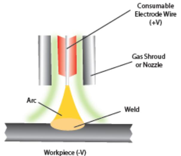
The electrode MIG gun is normally +VE and the work return is normally -VE. However, certain consumable wires sometimes require what is called reverse polarity i.e. Electrode -VE work +VE. Typical of these types of wire are cored wires used in hard facing or high deposition and gasless applications.
