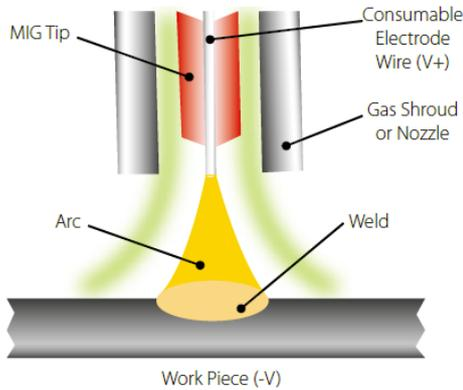
MIG welding was developed to help meet production demands of the war and post war economy which is an arc welding process in which a continuous solid wire electrode is fed through a MIG welding gun and into the weld pool, joining the two base materials together.
