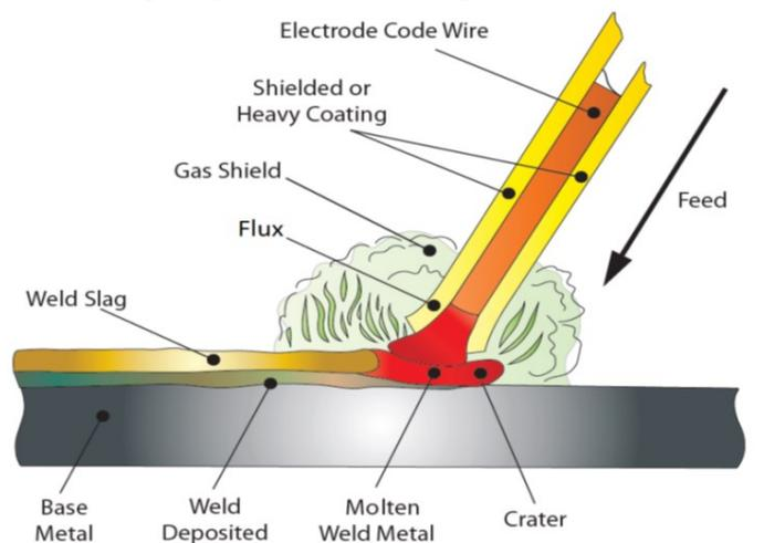
When the electrode is moved along the work piece at the correct speed the metal core deposits a uniform layer called the weld bead.
