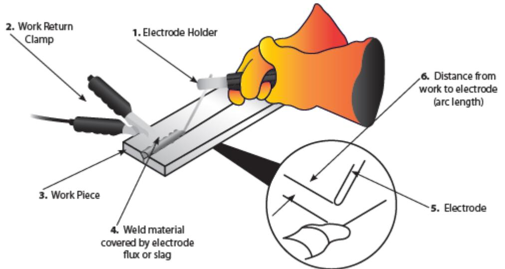
Welding current will flow in the circuit as soon as the electrode contacts the work piece. The welder should always ensure a good connection of the work clamp. The nearer the clamp is placed to the welding area the better.
