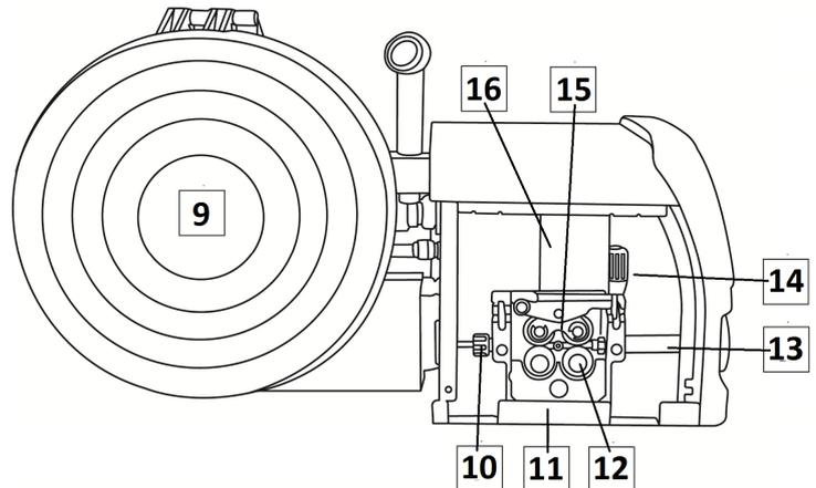
\* On the latest Wire Feed Units, the welding cable connects to the feed unit via a welding lug, where as older feed units (as shown above) used a Dinse plug/socket arrangement.
