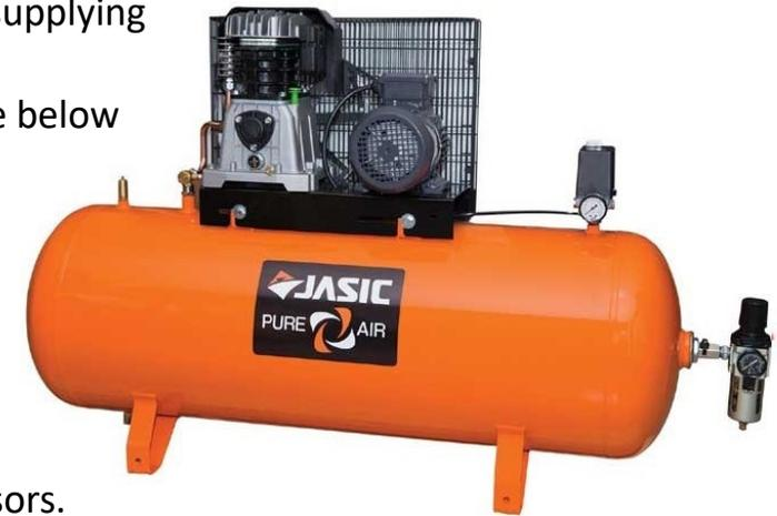
The accessories used with the compressor are also important, providing the correct air pressure, air flow which is moisture and oil free is crucial in ensuring that your plasma will give you quality cuts.
